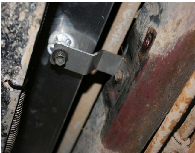
Above –Detail of position holes to be made for pipe routing. Below – Bracket mounting detail.
