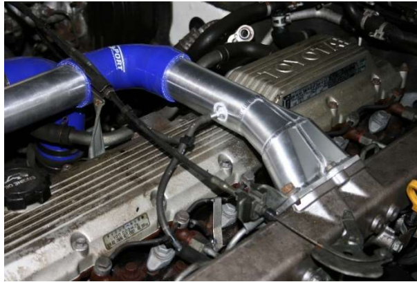
Above - 12 valve HDJ80 fitted with AlliSport manifold adaptor. 24 valve also available, kit fitting is identical
