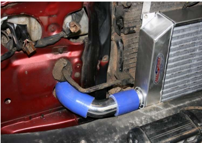
Above –Detail of position holes to be made for pipe routing. Below – Bracket mounting detail.
